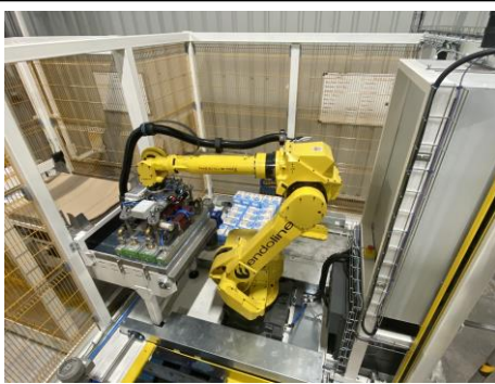
Image 1: The Fanuc M710 robot has enabled Carr’s meet increased demand and manage the palletising of 167,000 bags of flour per week
