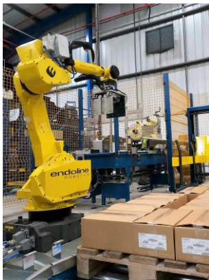
Image 1: Endoline’s robotic palletising solution features a FANUC M-710C/70 arm and a bespoke mechanical gripper to guarantee the reliable pick of every box
